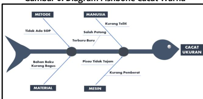
Gambar 7. Diagram Fishbone Cacat Ukuran
