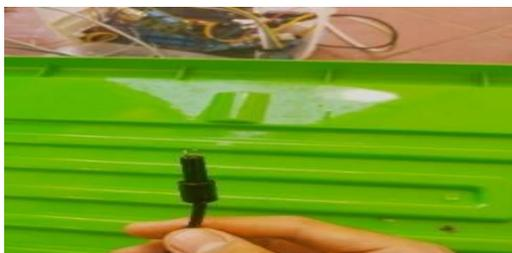
Gambar 1. Probe Sensor TDS
